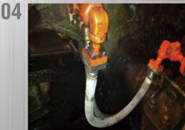
Swivel Joint connects with flexible hose
