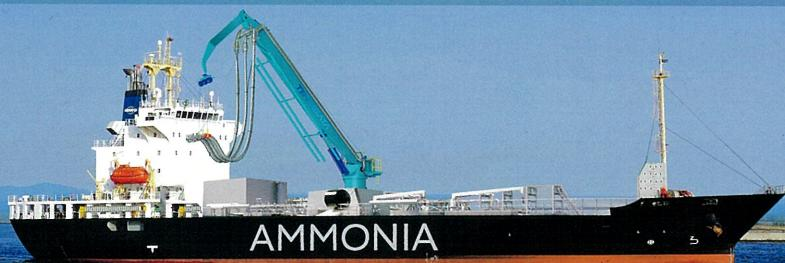
The bunkering boom, featuring a combination of rigid pipes, swivel joints, and hoses, has received Approval in Principle (AiP) from the classification society ClassNK, marking a significant step toward the safe adoption of ammonia as a marine fuel.
