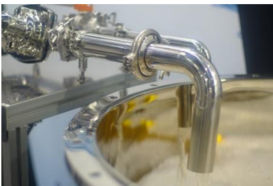
Swivel joints of various shapes and sizes are available for flexible piping.
