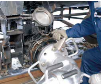
■ Cross-Over Bottom Connection to bulk tank simultaneously for loading multi-application.
