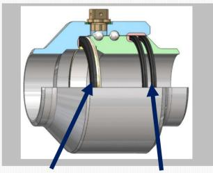
Special Main packing (For internal pressure)
