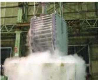
Cryogenic temperature test for LNG Butterfly Valves
