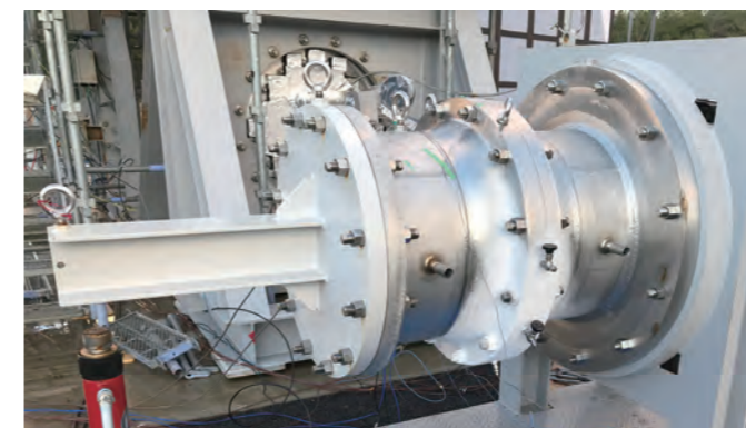
16" Ship Shore Coupling (SSC) tested by LH2
